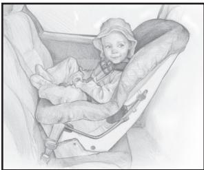
**Figure 3.** Convertible car safety seat used rear-facing.
